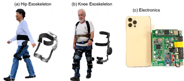
Fig. 1. (a) Our hip exoskeleton has high torque capability while providing optimal comfort and compliance. (b) Our lightweight knee exoskeleton is designed to enhance mobility and provide support for different activities while remaining compliant. It can also integrate with the hip module. (c) Our compact electronics architecture enables simultaneous control of our hip and knee exoskeletons, enhancing their coordination and functionality.
